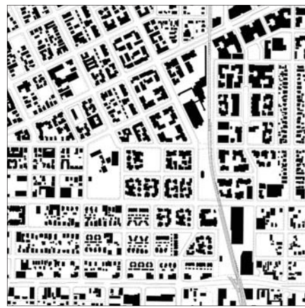
Building Positive Diagram of Traditional Neighborhood Development: Walkable, and Small Interconnected Network of Blocks and Multi-modal Streets
